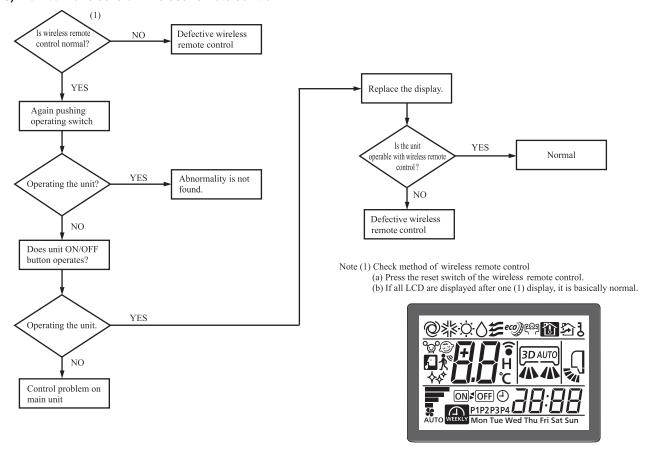
Simplified check method of wireless remote control
